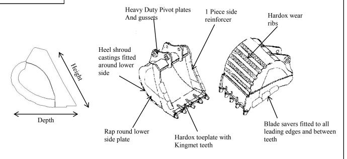
Buckets 54" or wider are also fitted with a shallow centre rib (not shown)
